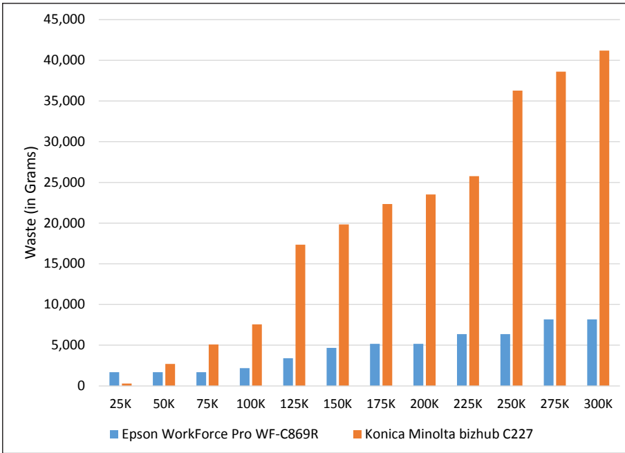
This graph shows the cumulative weight of waste consumables and packaging generated over the course of the 300,000-impression test run, with weights plotted at 25,000-impression intervals.
